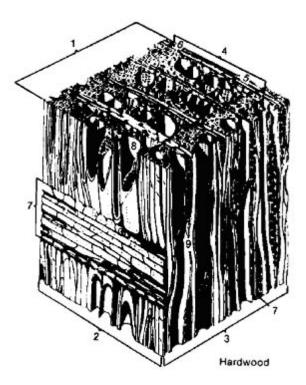
Figure 1-4-Wood structure of a hardwood. (ML88 5570)
