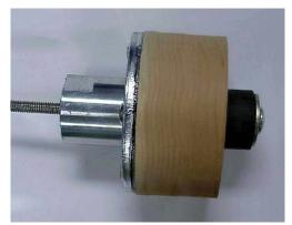
I have a hand-wheel on my lathe, and the center is tapered slightly. I turned a wooden plug to fit that taper, and extend out about a ½". The threaded rod should be just long enough to pass through this plug by about a ½ to ¾" when the compression plug is "uncompressed". The faceplate and plug are center bored for the diameter of the threaded rod, centering the compression plug when in use. A threaded knob is threaded on the rod as it extends through the handwheel side tapered plug.
