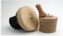
Smaller-size shopmade screw chucks provide fast and easy mounting of small projects such as chessmen (right). Use a lag bolt if more support is needed, as shown in the example on the left that uses a faceplate and a scrap of plywood.
