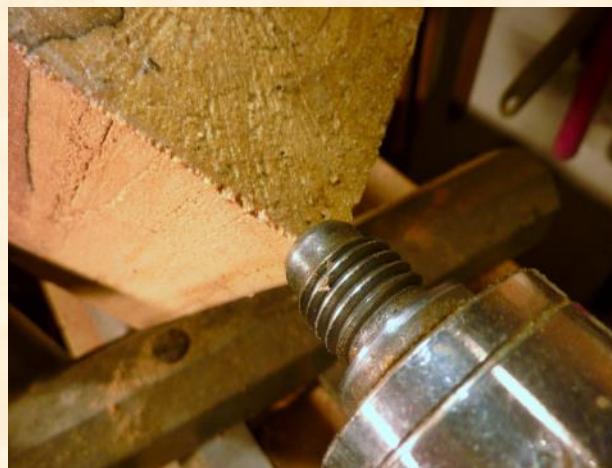
Figure 2: Cube secured in Hollow One-Way live center
