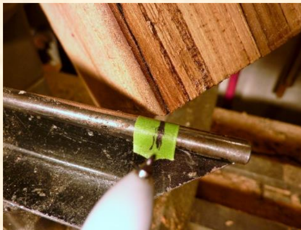
Figure 3: Mark the location where the cube corner swings past the tool rest
