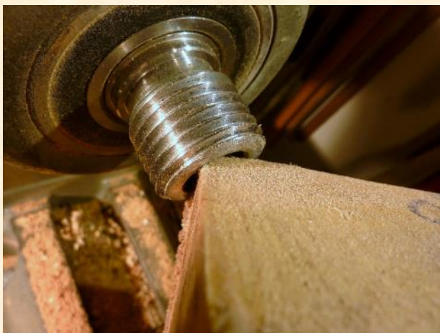
Figure 1: Corner inserted in Hollow Spindle
