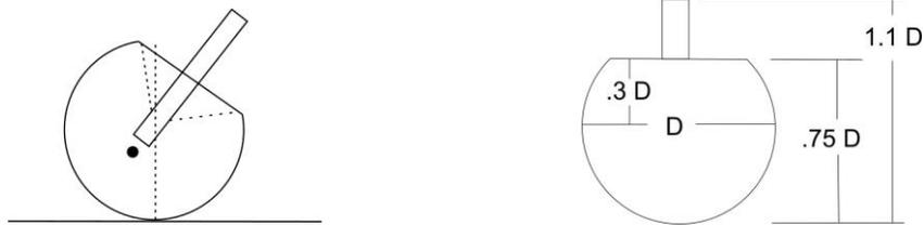
1. Start with a blank that is approximately 1.5 inches square and at least 2 inches long. Turn it round at somewhere between 1 and 1.5 inches, turn a tenon to fit your chuck and mount the blank on the chuck. In the diagram above, D is the diameter and the other dimensions are based on D. For example the height is 0.75 times D (or  $\frac{3}{4}$  D).
