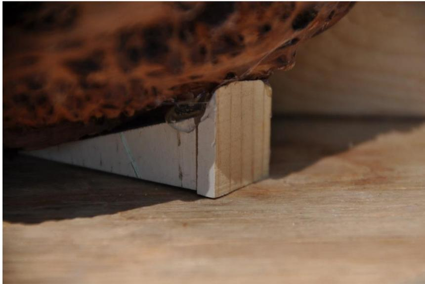
Continue to build the wedge. Don't go all the way to the edge of the burl, otherwise truing up the face could start cutting the wedges.
