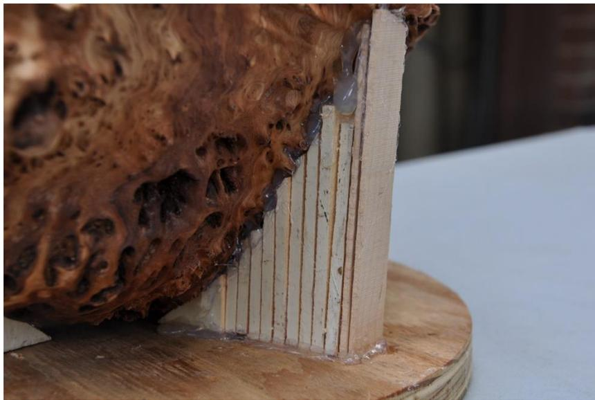
Keep building wedges. Once the second one is started, you should be able to remove the temporary 2x4 wedges. I build at least 5 wedges.
