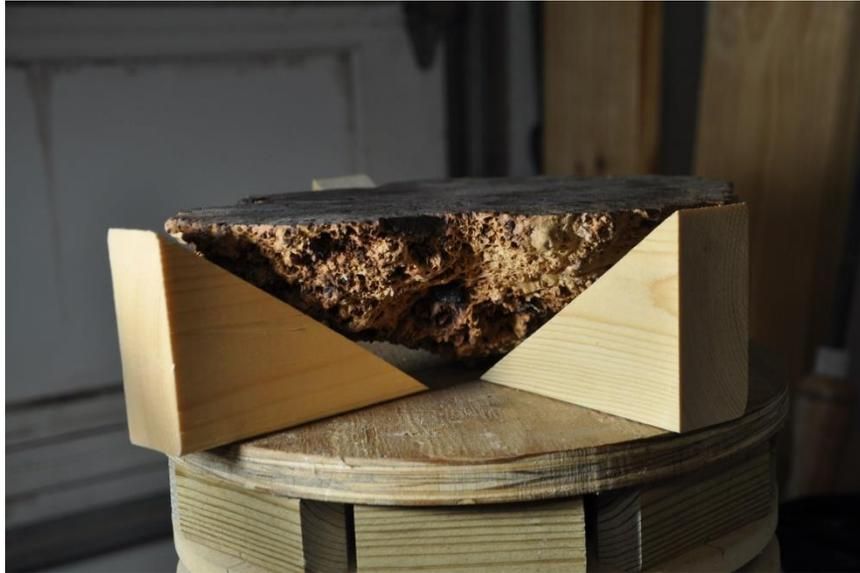
Measure the maximum height from the plywood to the burl. Cut \*lots\* of thin strips of scrap wood of varying lengths, no longer than the maximum height. I usually cut several pieces from the end off of a  $\frac{3}{4}$ " pine board at a slight angle and slice it thinly with a bandsaw. Cut the strips with the grain. Save the small wedges at the thin ends to start the gluing process.
