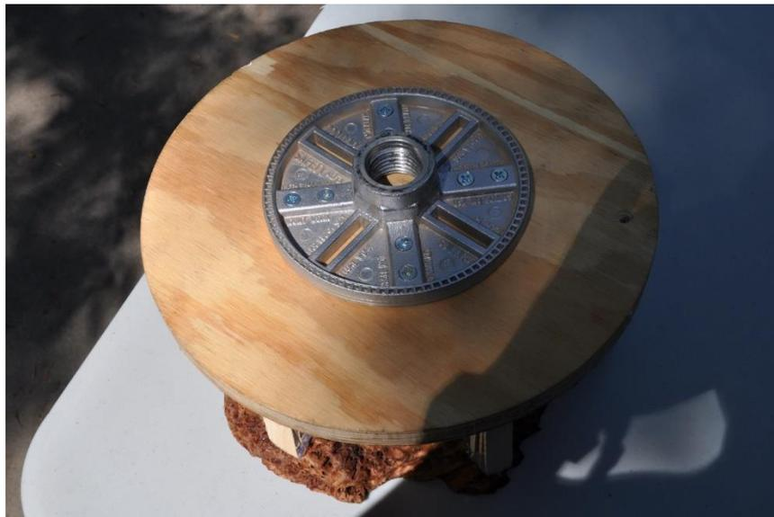
Mount it on the lathe. Use the opportunity of this new perspective to fill in the gaps in the glue between the wedges and the burl. Put a bead of glue around the base of each wedge.
