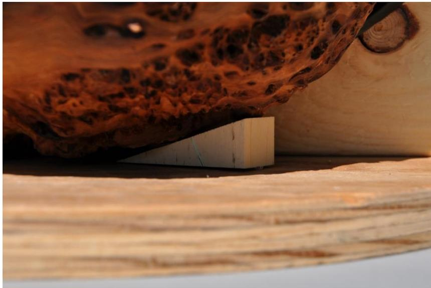
Continue to build the wedge using the thin strips. The wedge should conform to the surface of the burl as much as possible. I use a sanding disc to tweak the length and shape of each strip as necessary. Glue each strip to the piece that came before it, as well as the plywood and the burl.
