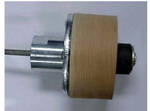
I have a hand-wheel on my lathe, and the center is tapered slightly. I turned a wooden plug to fit that taper, and extend out about a ½”. The threaded rod should be just long enough to pass through this plug by about a ½ to ¾” when the compression plug is “uncompressed”. The faceplate and plug are center bored for the diameter of the threaded rod, centering the compression plug when in use. A threaded knob is threaded on the rod as it extends through the handwheel side tapered plug.
