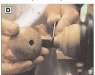
After turning the interior, use the spindle gouge to continue refining the shape of the globe. Don't forget that you have a 3/8" hole drilled through the entire globe. When you are satisfied with the shape of your ornament, sand the globe, apply sanding sealer, and part it from the lathe as shown in Photo D.
