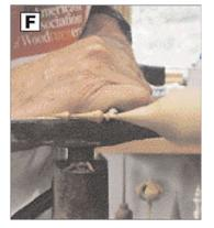
Next, use the roughing out gouge to start turning the icicle. You won't have the support of the tailstock to rely on, so take light cuts. I turn the smallest segment first (the tip of the icicle). I reduce the diameter with the roughing out gouge, and then refine the shape with a small skew and small spindle gouge as shown in Photo F.
