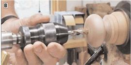
As you turn, clean out the shavings; if they build up too much, they can grab the tool and destroy the globe. (The shavings build up more with green wood than dry wood.) Compressed air is one solution, but if you don't have a compressor, a small piece of plastic hose or straw will suffice to blow out the shavings.
