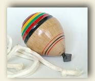
We are going to concentrate on the basic spinning top. Making a spinning top on a lathe is nothing more that spindle turning with the grain of the wood running parallel to the lathe bed. There is no one design; tops come in all shapes, sizes and material. Our goal will be to make a top that will spin for at least 60 seconds.
