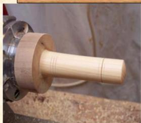
In this photo, the outside of the needle case has been turned and it is ready to part off just in front of the disk holding it in the chuck.
