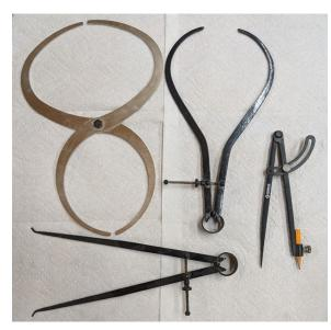
Internal, External and Thickness calipers. Compass for marking OSB stock for ring cutting
