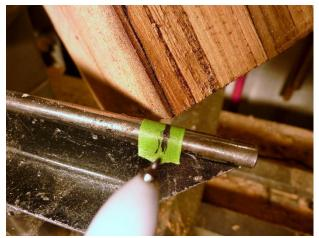
Figure 3: Mark the location where the cube corner swings past the tool rest
