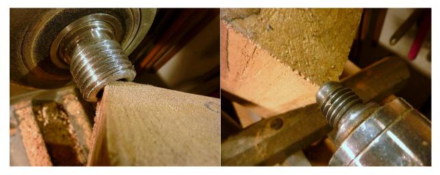
Figure 1: Corner inserted in Hollow Spindle
