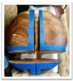
**13.** Remove painter's tape and finish the new unfinished wood surfaces by sanding, clear stain and then several coats of polyurethane. I found the use of painter's triangles extremely helpful when finishing with the polyurethane coats.
