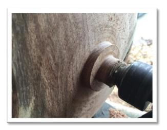
**5.** Remove from lathe, remove face plate, reverse piece and mount it back onto lathe with tenon in chuck.
