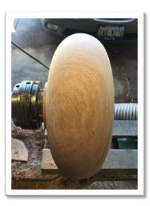
**6.** Once finished turning and while still on the lathe, sand as needed and desired.
