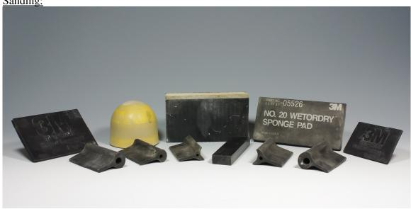
In some ways this is the most important part of a good finish. Sanding is where a good finish is made or lost. I will start with the finest grit possible and it really depends upon how heavy the ridges are on the surface. As mentioned before, the ridges are caused by the centrifugal force of the piece as it spins. These bumpy rings need to be flattened or leveled. Both dry and wet sanding can and are employed in this step of the finishing process.
