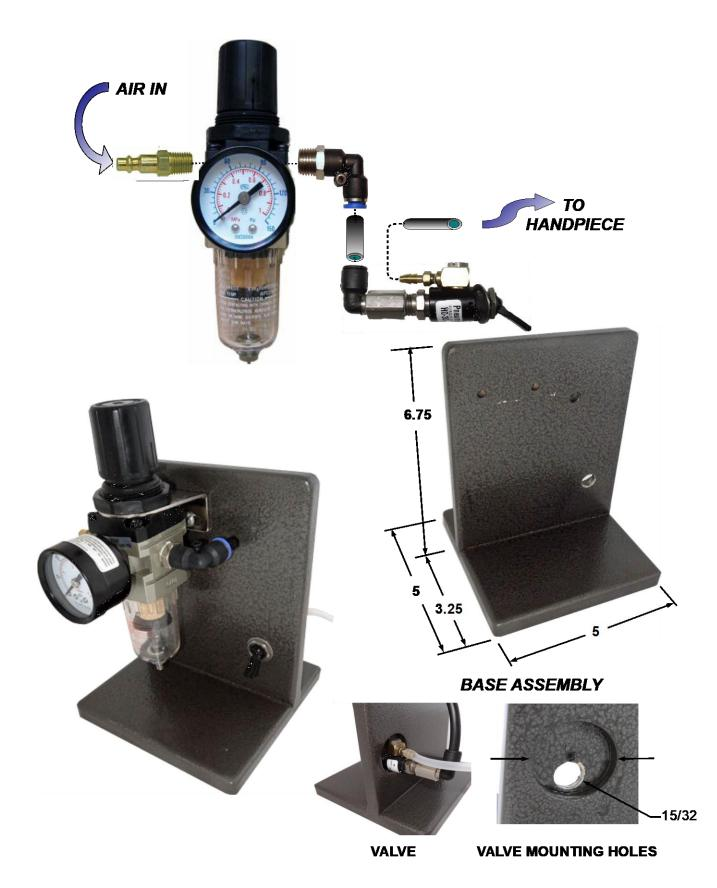
Use Teflon plumbing tape on all of the pipe threads. Be extra careful not to get any of the tape onto the face of the fittings as it can come loose and get into the turbine slots. Two clockwise wraps of tape around the threads is proper. The rigid tubing fittings are push type which only require you push the tube into the fitting and pull it back to engage the lock. If you need to remove the tube just compress the locking ring and pull the tube out.
