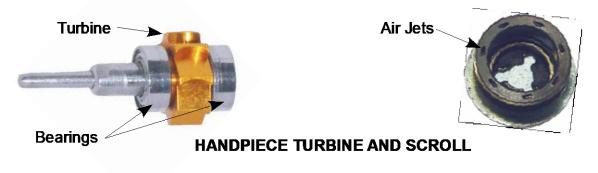
A compressed air source is required. The handpieces only require about 2 CFM of air volume at 45 PSI. A compressor rated at 3 CFM at 60 PSI will work, but larger is better. The higher the volume the less cycling will occur. If you don't already have an air compressor, an inexpensive "pancake" unit will work fine. A moisture separator on the compressor is very desirable.
