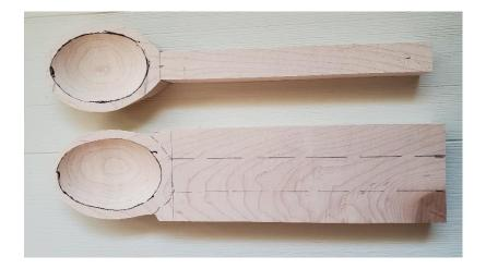
Mount one spoon on the lathe using a small steb or spur drive and the live center attachment in
