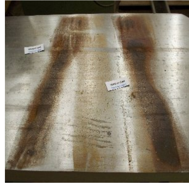
Tannin damage to cast iron jointer table.
