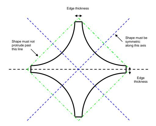
I always use ¼ circles for the curves, but any shape can be used as long as it's symmetric along the blue diagonal axes and does not protrude past the green lines. The same shape must be cut on both sides.
