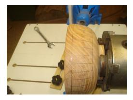
Set up the Flute Master – Index Wheel – Index Pin Holder -Stop Blocks – Flute Depth. I always check the number of flutes by using the table and then drawing the flutes on the piece. Just me!
