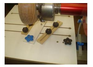
Platform Holders - Used to hold the platform to the lathe
