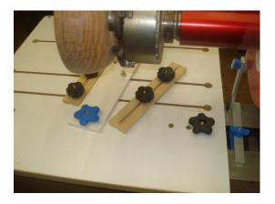
Begin cutting flutes. Make sure that when moving the router that you stay on path. Start at the top and go to bottom. Move the stand to the inside stop block and then it will swing correctly and give a good cut. Doing is the only way to get this done on a consistent level.
