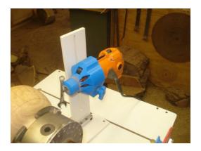
Set the inside stop block by aligning the router and stand to the inside line. Then move the stand and router to the outside line and set stop block. This will assure that all your flutes will be the same length
