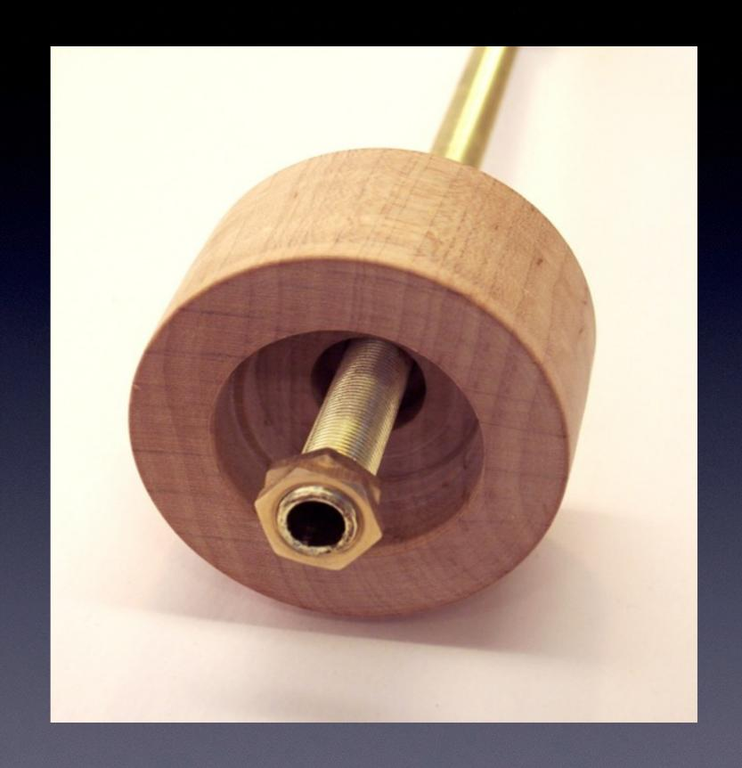
Complete Bearing adapter with one bearing
